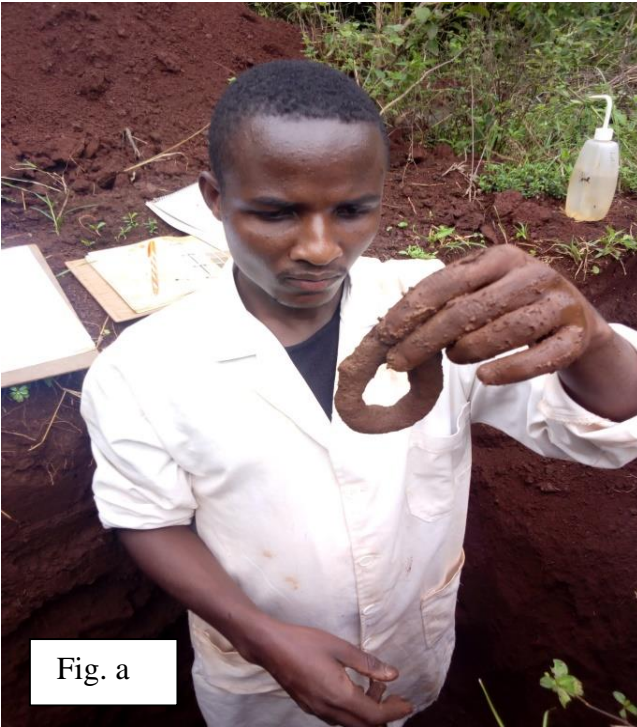
Testing soil plasticity (Figure a) and identification of profile horizons (Figure b).
