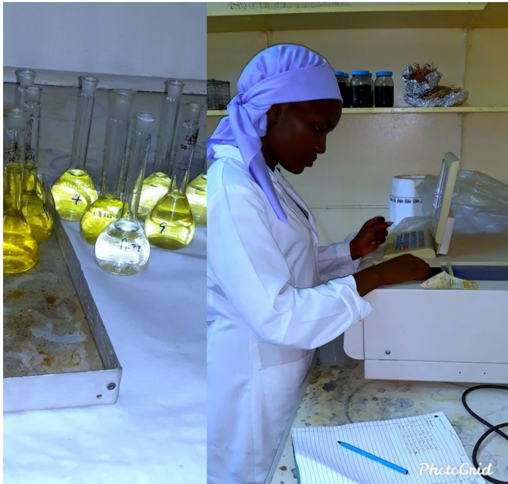
Plate 3.3: Researcher analyzing for phosphorus using the calorimetric method at the University of Nairobi
