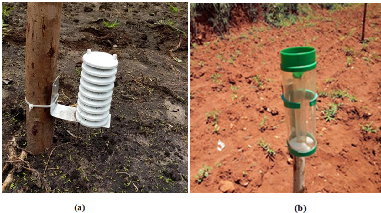
Figure 3: Equipment deployed in the farms (a) Temperature logger and (b) Rain gauge
