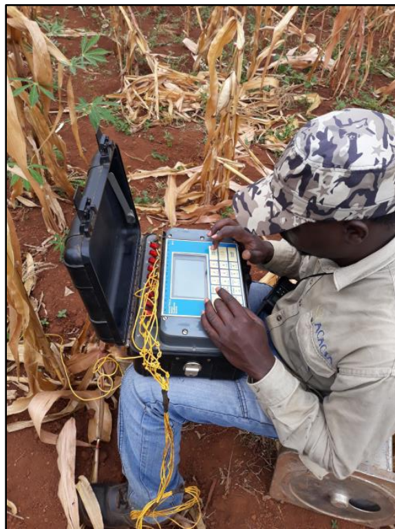
Figure 3.15: Measurements of gradient IP using the IPR-12 receiver.
