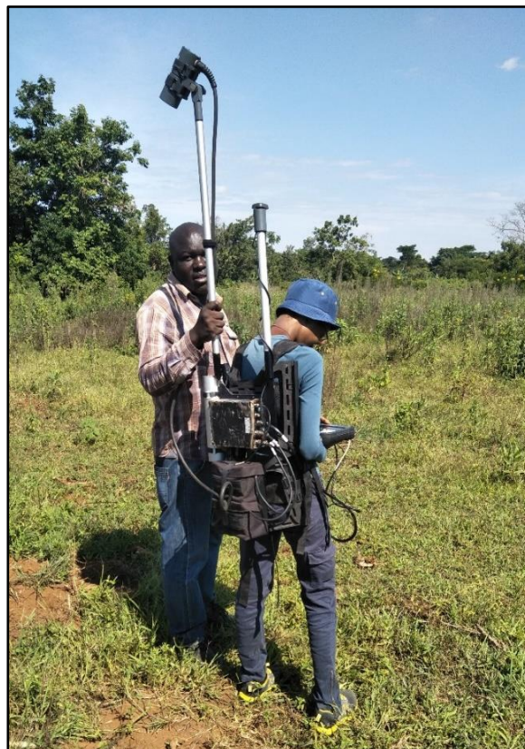
Figure 3.21: Field operation of the Envi-Cs Magnetometer during magnetic survey in Makina
