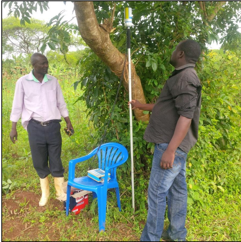
Figure 3.22: Setting up of the Base station Envi-mag (BaseMag).
