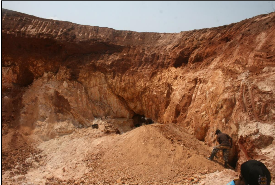
Figure 2.10: Artisanal mining site in Makina. (Note thickness of the weathered overburden encountered in most parts of the prospect).
