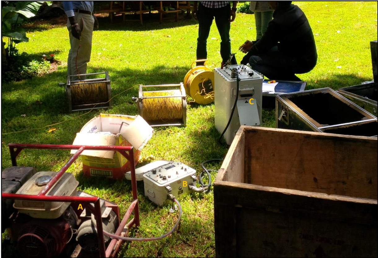
Figure 3.17: Typical set up of the current transmission station; A- Generator, B- Voltage regulator, C- Zonge GGT-3 transmitter.
