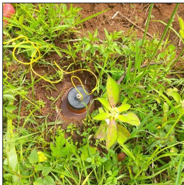
Figure 3.12: Potential measurement line laid out during gradient measurements.
