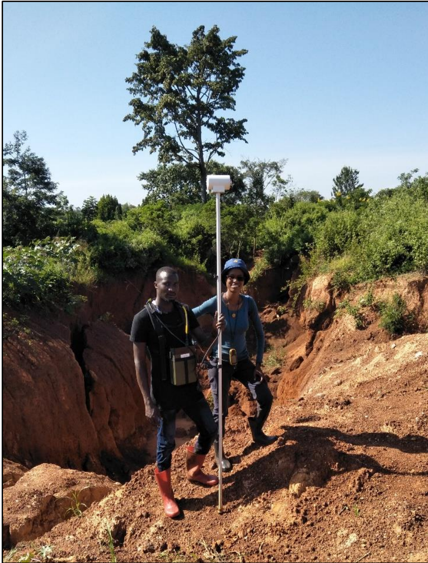
Figure 3.20: Magnetic surveying using the Geometrics, G857 Proton Precession Magnetometer.
