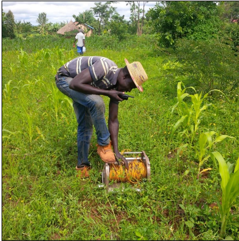
Figure 3.10: Photo showing laying out of the measurement lines during the gradient survey.
