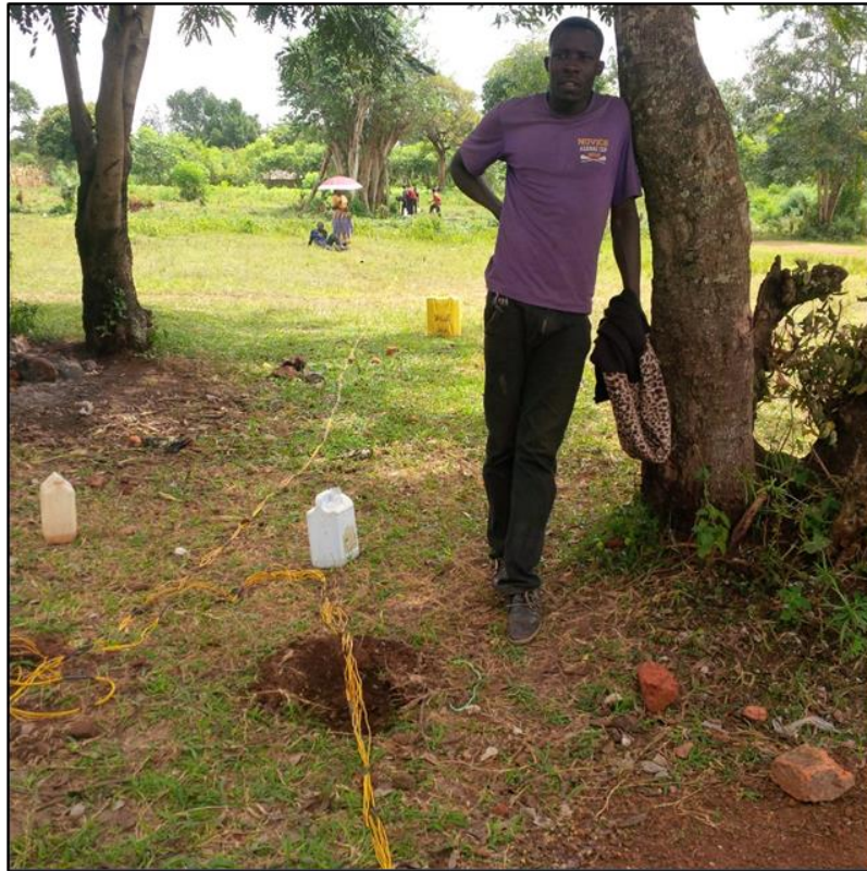
Figure 3.12: Potential measurement line laid out during gradient measurements.
