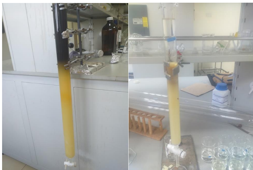
Figure 3.2-4: Column chromatography of the studied plant fractions
