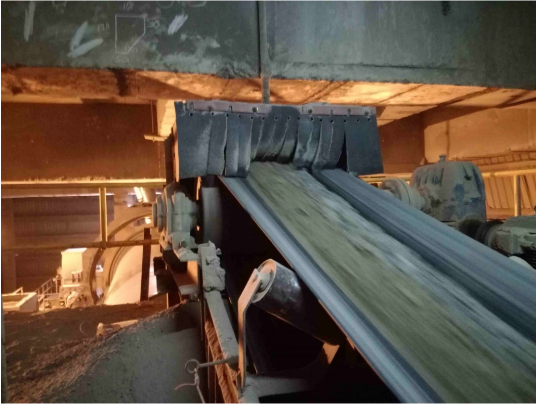
Figure 3.7: The point of introduction of the tracer - the conveyor at the inlet of the ball mill
