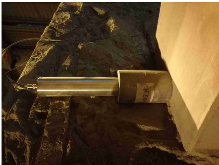
Figure 3.9: Detector D3 with a lead collimator at the recycle line from the separator
