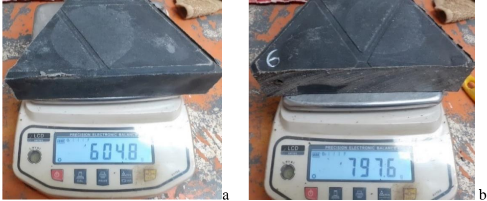
Plate 3-9: After the test the specimens are weighed to obtain M_2
