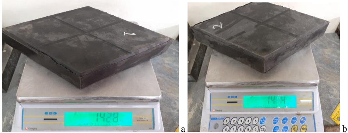
Plate 3-5: The submerged samples are weighed to obtain M_2
