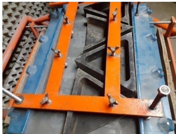
Plate 3-8: The specimens fastened on the tumbler machine
