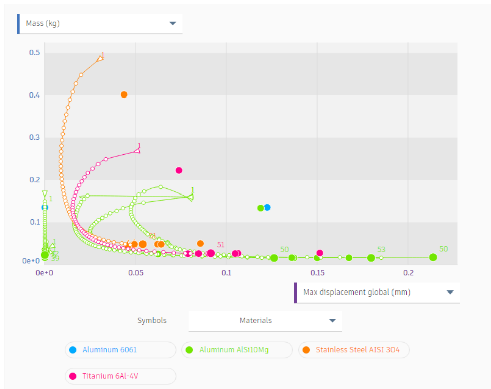
Figure 16; Results dispersion graph produced by the GD exploration environment, mass vs max displacement, solutions grouped according to the material.
