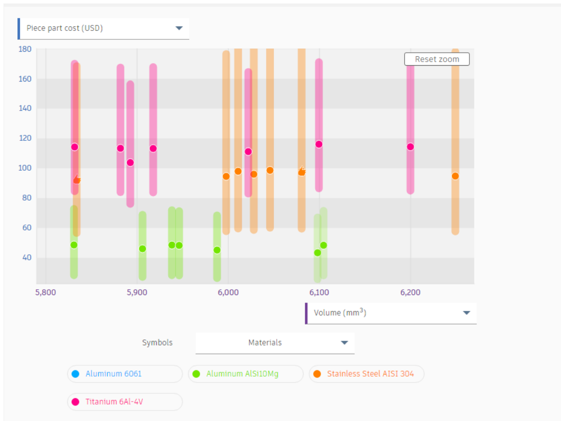
Figure 19 Results factor of cost produced by the GD exploration environment, cost in dollars vs total volume, solutions grouped according to the material
