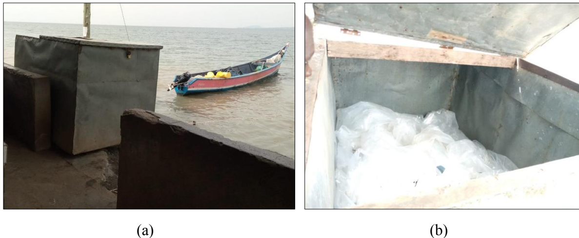
Figure 5.3: Locally fabricated cooler boxes for fish (a) External view and (b) Internal view.
