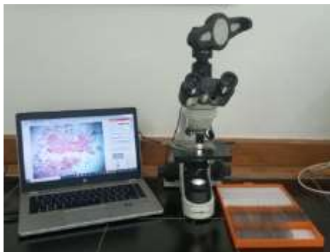
Figure 10: Richter Optica Achromatic Plan XU-T1 digital microscope interphased with Moticam BTU 10 Camera systems connected to a computer with the Motic Images 3.0 software open
