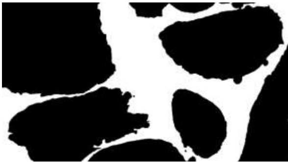
Figure 10: Image in figure 2 segmented using the auto threshold method to enable measurements by FIJI/Image J
