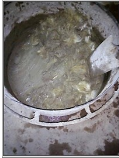
Figure 3.9: Image showing 30 mm chopped sisal fibre mixing with OPC mortar in the cement mixer at the Concrete Laboratory, UoN.
