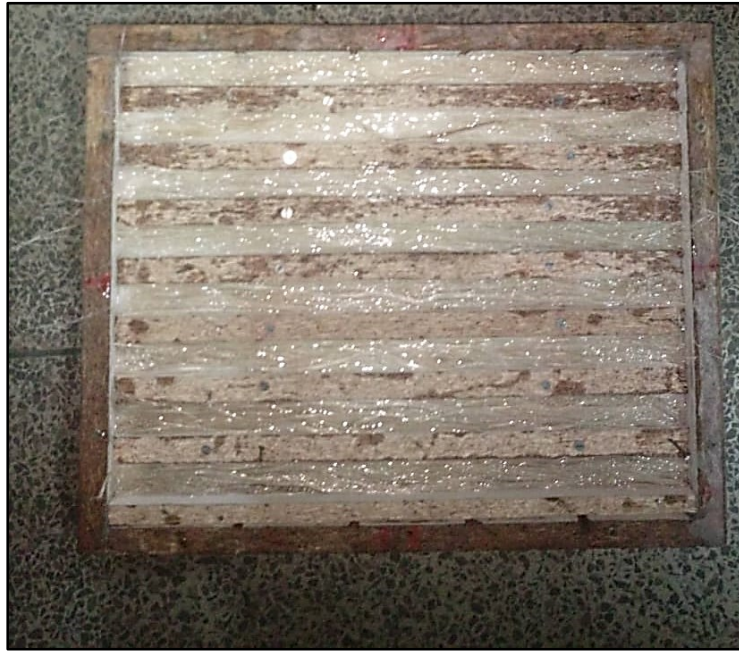
Figure 3.12: Image showing cured polyester resin specimens in mould ready for demoulding
