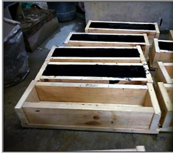
Figure 3.8: Image showing well-oiled flexural specimen wooden moulds at the Concrete Laboratory, Mechanical Engineering building, UoN
