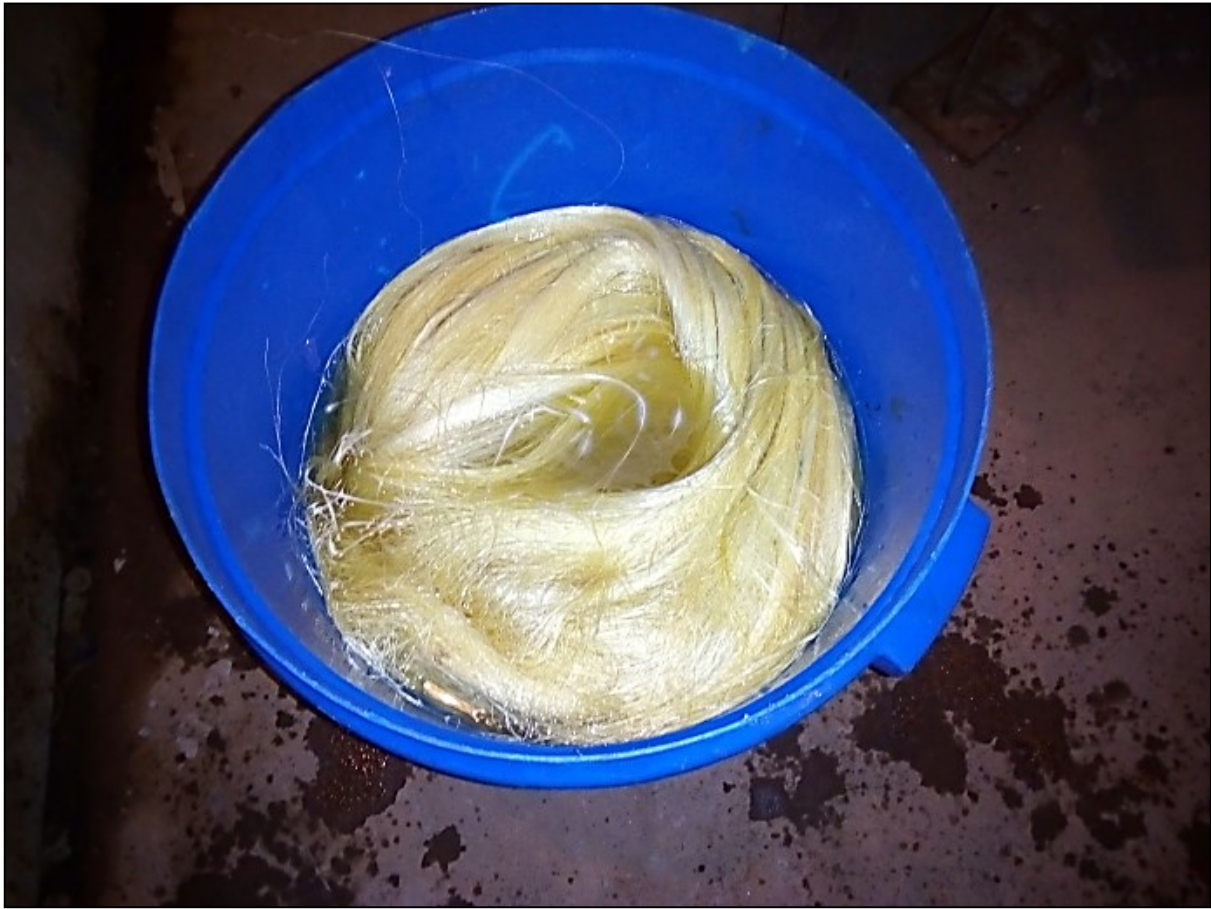
Figure 3.1: Image showing sisal fibres mercerising in a 0.06M NaOH solution.
