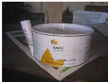
Figure 3.14: Image showing KAPCI polyester putty and dibenzyl peroxide hardener used in the study
