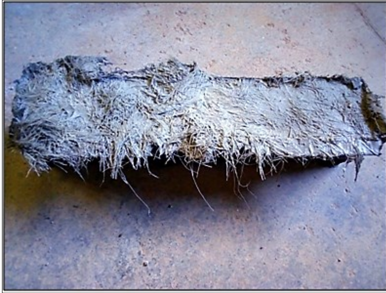
Figure 4.12: Image showing fibre clumps on a 7% randomly oriented discontinuous fibre-reinforced mortar surface.
