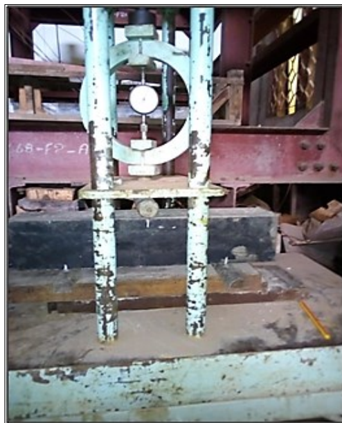
Figure 3.17: Image showing 3-point bending test on a fibre-reinforced OPC mortar specimen in progress on a bending and transverse testing machine at the Timber Laboratory, UoN.
