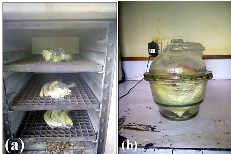
Figure 3.4: Image showing absorbency specimens in (a) convection oven and (b) desiccator jar before weighing.
