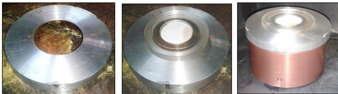
Figure 5.3: Part holding the sample above the radioisotope source and detector.
