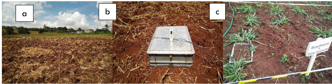
Figure 5. 2: The plots before planting. b) The complete set of static GHG sampling assemblage. c) The inter-row positioning of the static chamber in the field in newly planted Brachiaria plots (approx. two weeks old).
