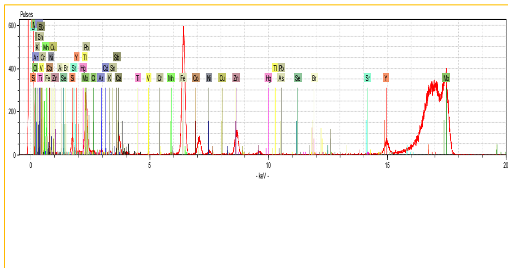
Figure 5 Spectrum of a Finger Nail Clippings Sample
