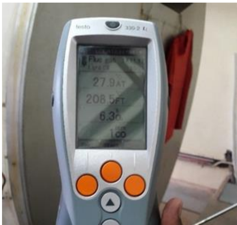
Figure 3-8 shows a magnification of the digital display of the flue gas analyzer in Figure 3.7
