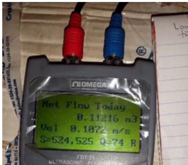
Figure 3-3 shows the magnified view of the ultrasonic flow meter
