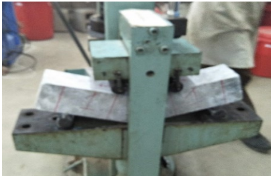
(a) Failure of prisms in flexure
