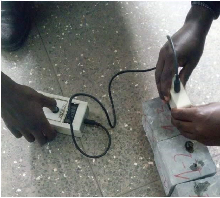
Figure 3.3: Electrical resistivity test in progress
