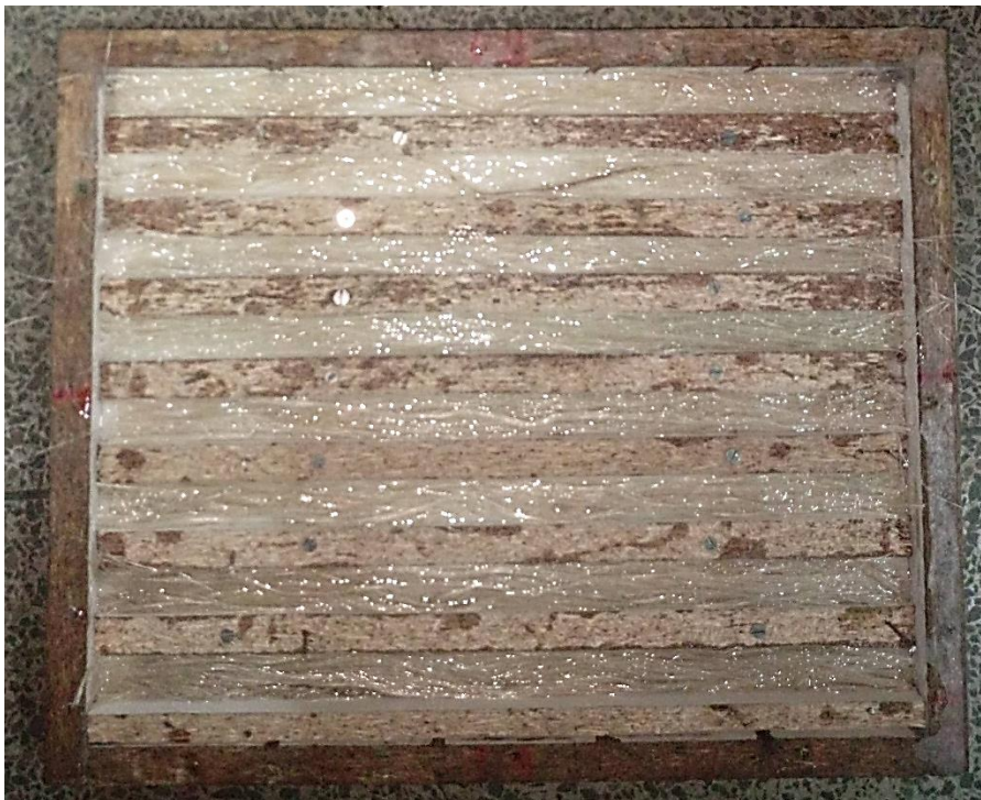
Figure 3. 11: Banana fibre-reinforced epoxy resin specimens ready for demoulding.
