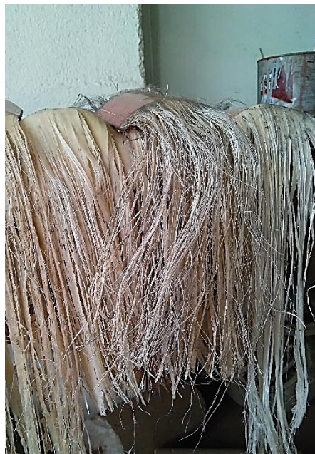
Figure 3. 4: Decorticated banana fibres that were used in the current study.
