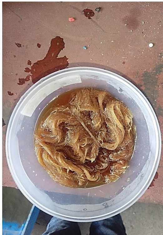
Figure 3. 6: Banana fibres mercerising in a 0.1M NaOH solution.
