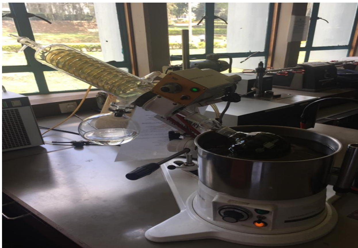
Figure 3.3: Photograph of a Rotary Evaporator. The picture was taken in the PHPT Laboratory of the University of Nairobi by Kevin Kariuki.
