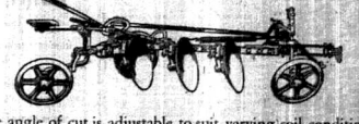
The angle of cut is adjustable to suit varying soil conditions, by means of a foot-rop wedge device.
