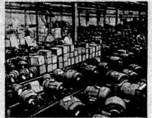
Dispensing conveyor in No. 1 works. 2000 motors per week can be handled in this section.
