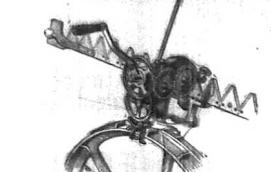
This inexpensive blade grinder is designed to meet the demands for a handy, portable machine with which the farmer can sharpen his mower knives easily and quickly...
