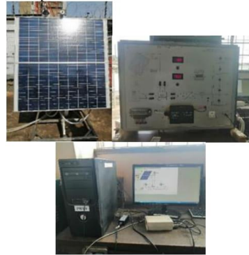
Figure 3: Solar PV trainer
