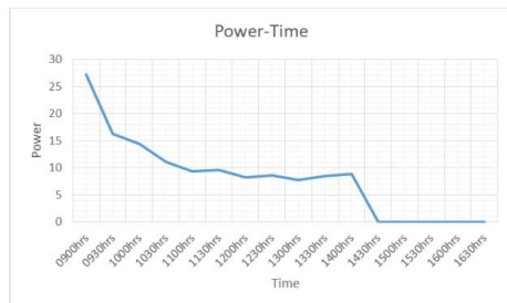
Figure 7: Power-Time graph at 14° tilt angle facing 278° West
