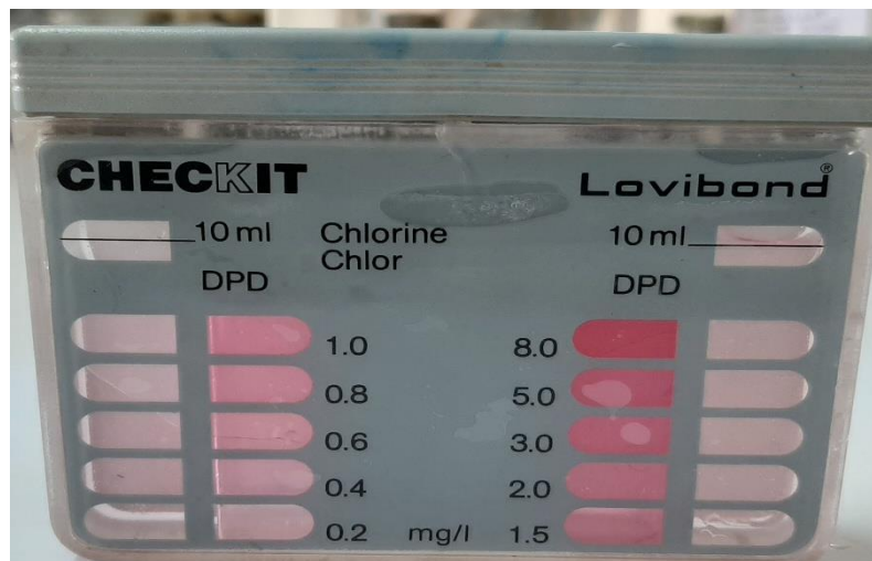
Figure 3. 8: Residual Chlorine analysis using LOVIBOND Chlorine (DPD) Checkit.
