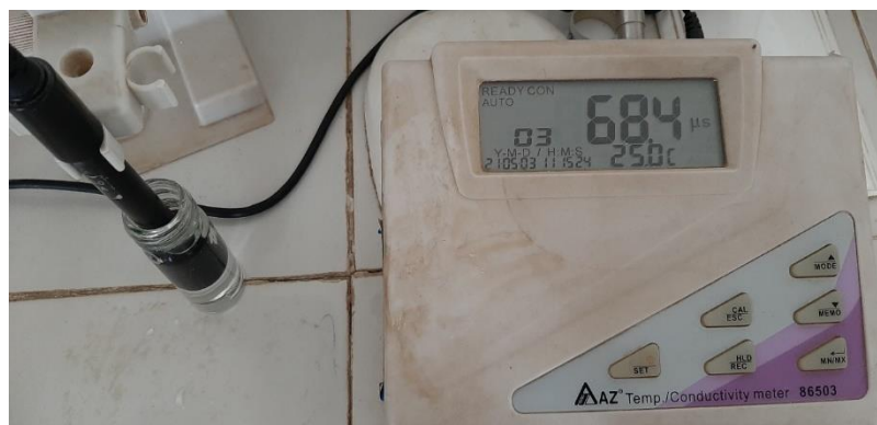
Figure 3. 5: Conductivity determination of water samples using a conductivity meter
