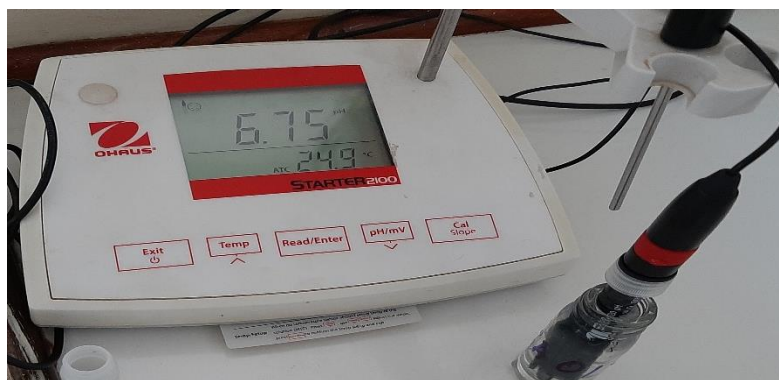
Figure 3. 4: pH determination of water samples using a pH meter
