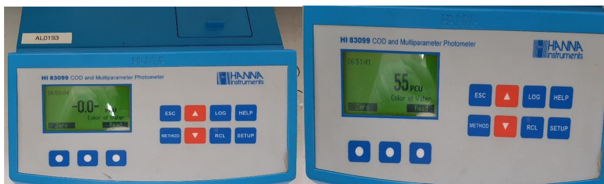
Figure 3. 6: Colour analysis of the water samples using Multiparameter Photometer.
