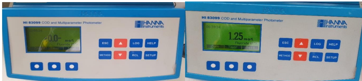
Figure 3. 7: Fluoride analysis of the water samples using Multiparameter Photometer.
