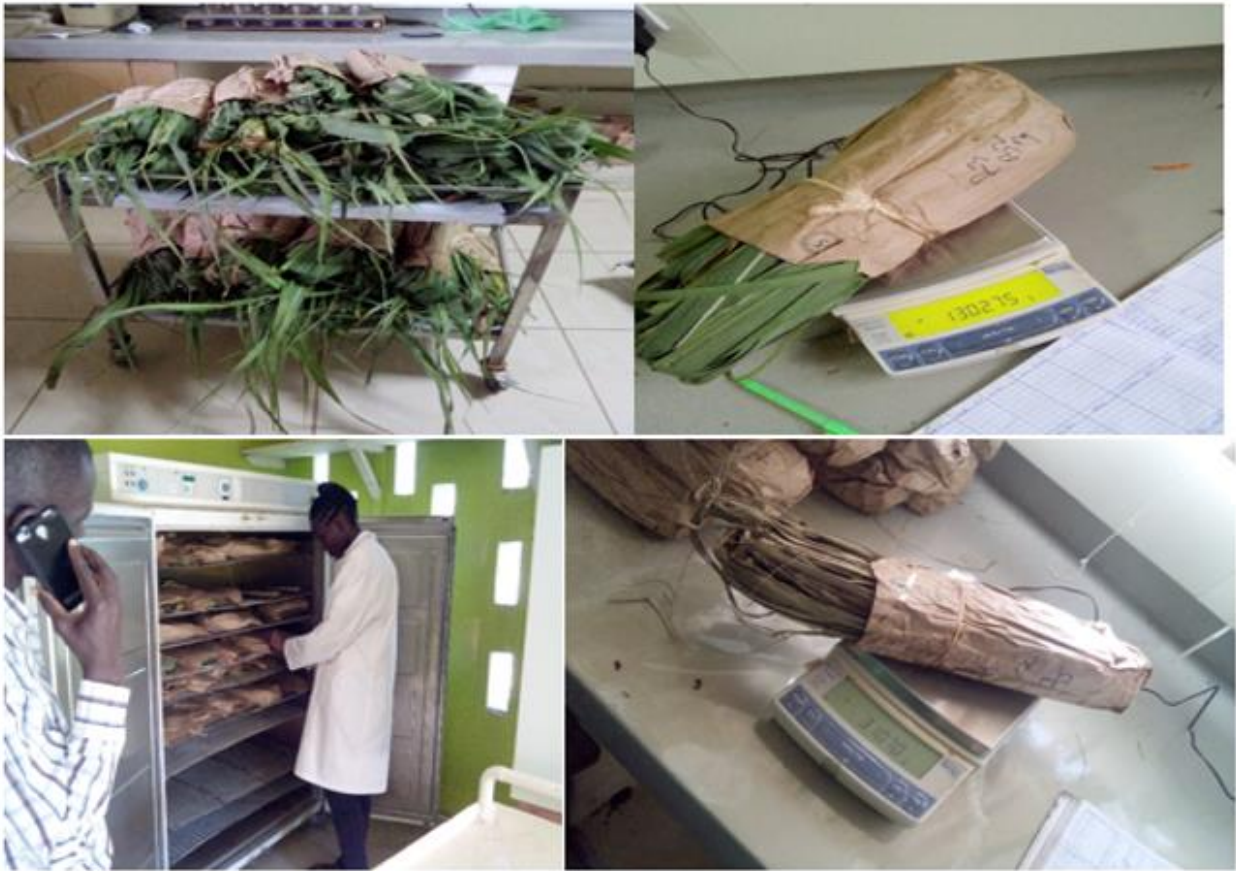
Sample collected, wet weighted, oven dried and weighted for dry mass
