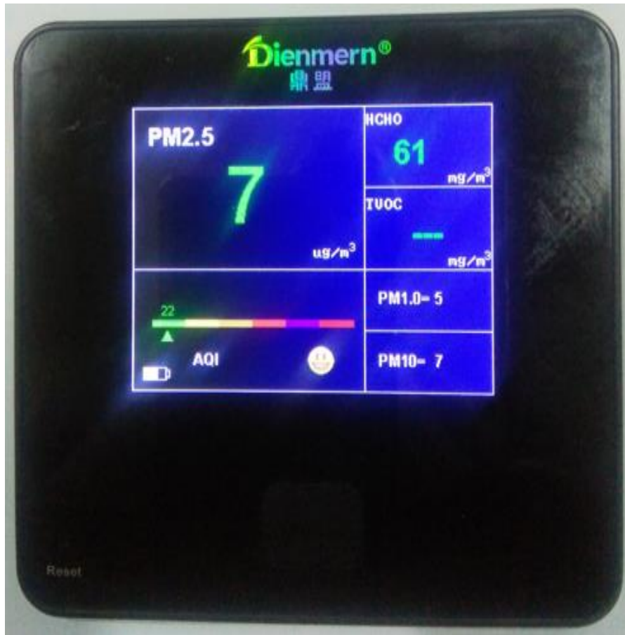
Plate 3.1: Equipment for measurement of particulate matter, HCHO and TVOC
