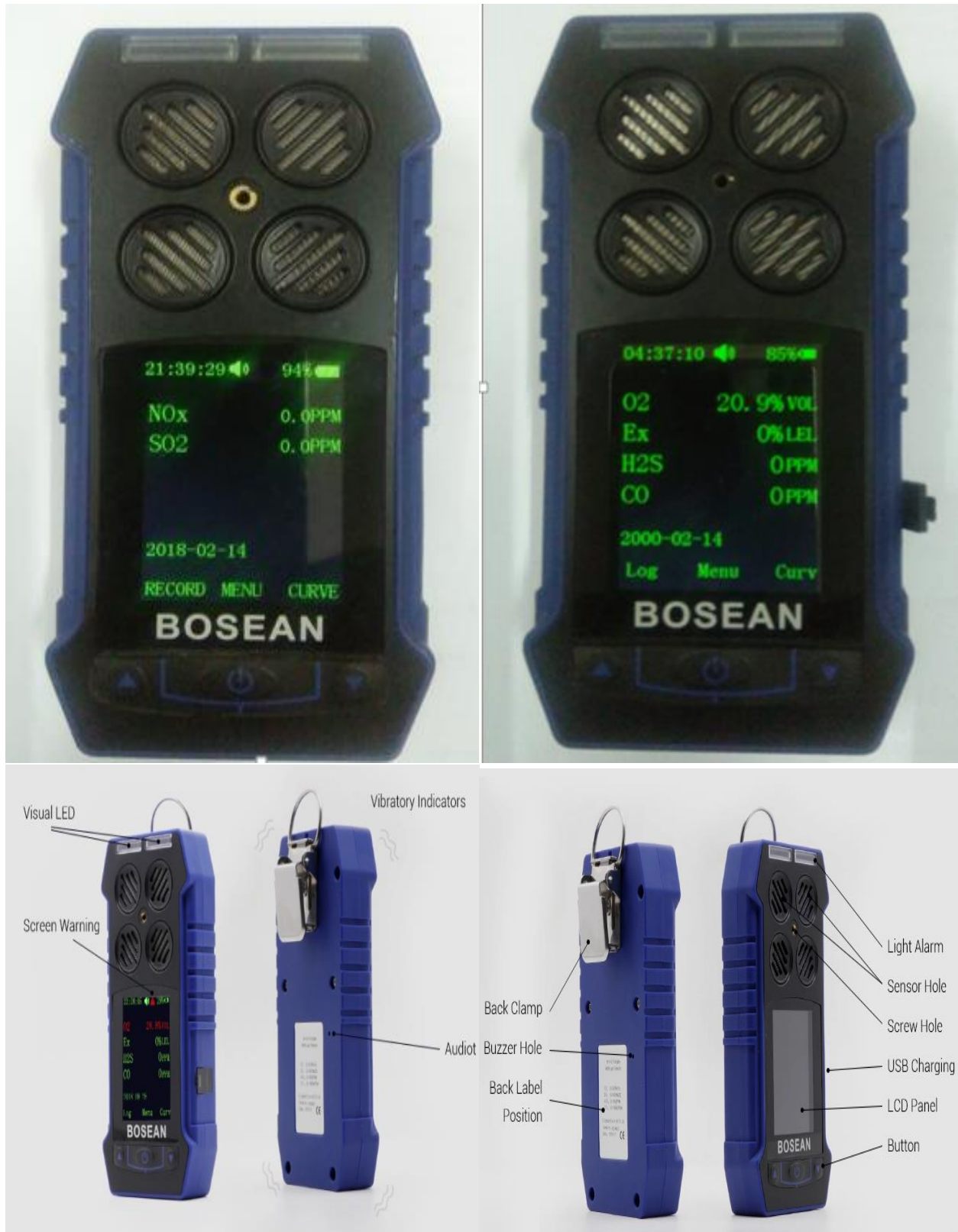
Plate 3.2: Equipment for measurement of Nitrogen oxide Sulphur dioxide, and Carbon Monoxide
