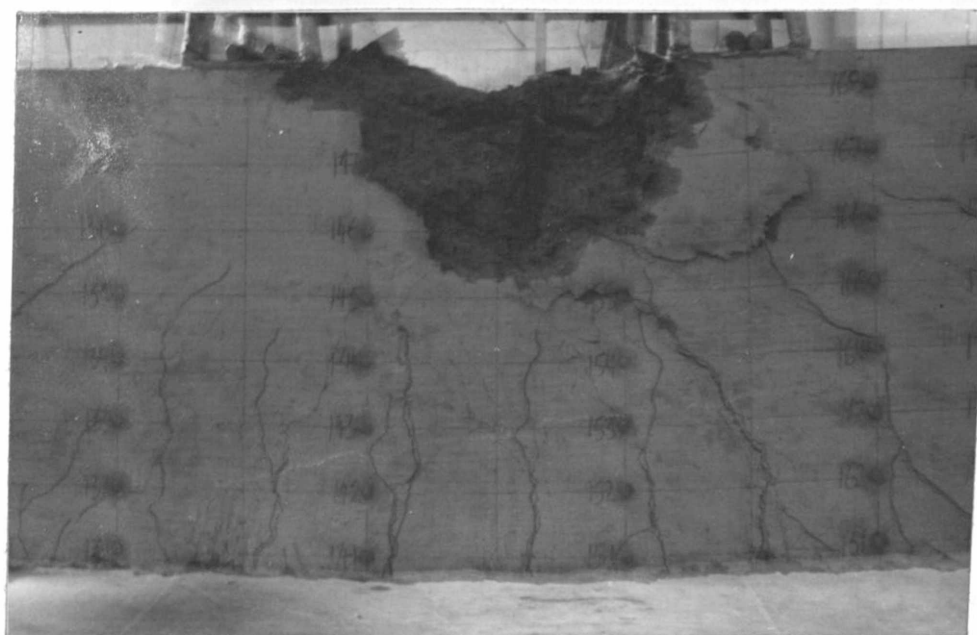
Plate C.4 : Failure , Beam CFT-TB 8
