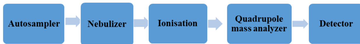
Figure 3.2: Basic illustration of Inductively coupled plasma mass spectrometer
