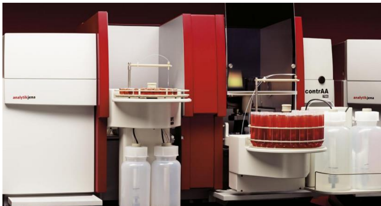
Figure 2.1: ContrAA 700 High Resolution Continuum Source (AAS) machine
