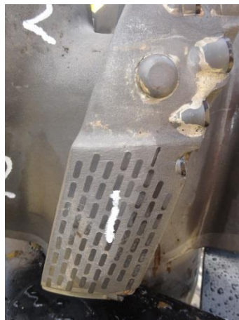
Fig 4.15: 12 1/4" SKHE616M Gauge View
