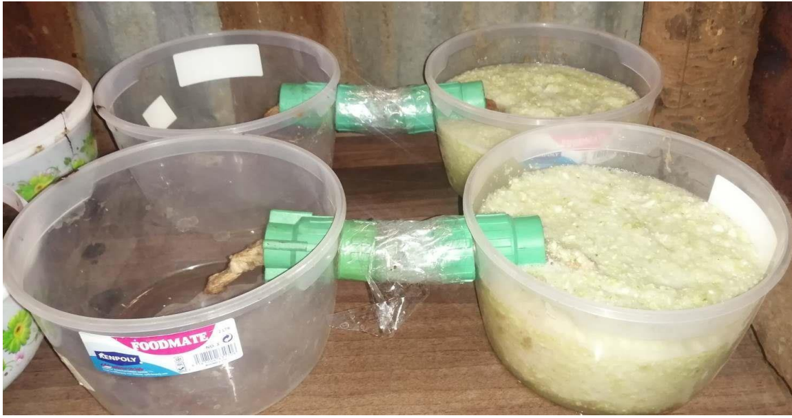
Figure 3.7: Microbial fuel cell control experiment setup with cabbage in the anodic chamber
