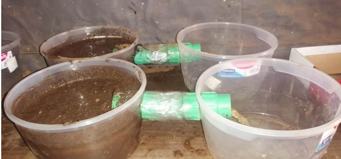
Figure 3.9: Microbial fuel cell control experiment setup with Loam soil in the anodic chamber
