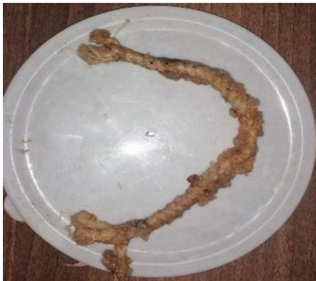
Figure 3.3: The wicks used to construct the salt bridge.
