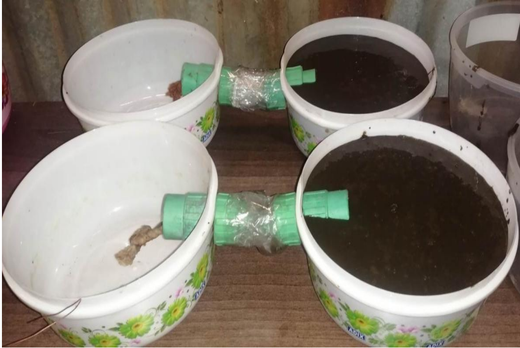
Figure 3.6: Microbial fuel cell control experiment setup with rumen in the anodic chamber
