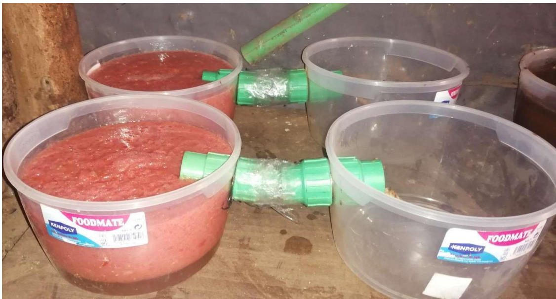
Figure 3.8: microbial fuel cell control experiment setup with tomato in the anodic chamber
