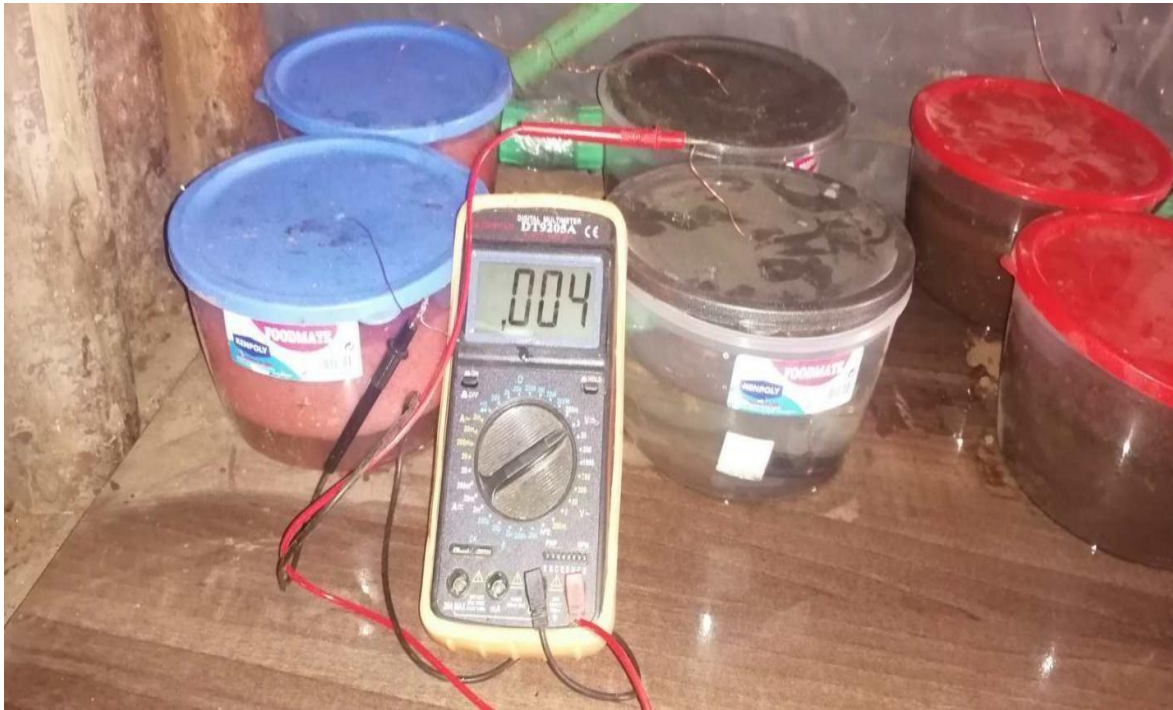
Figure 3.5: A multi-meter equipped twin cell (MFC)
