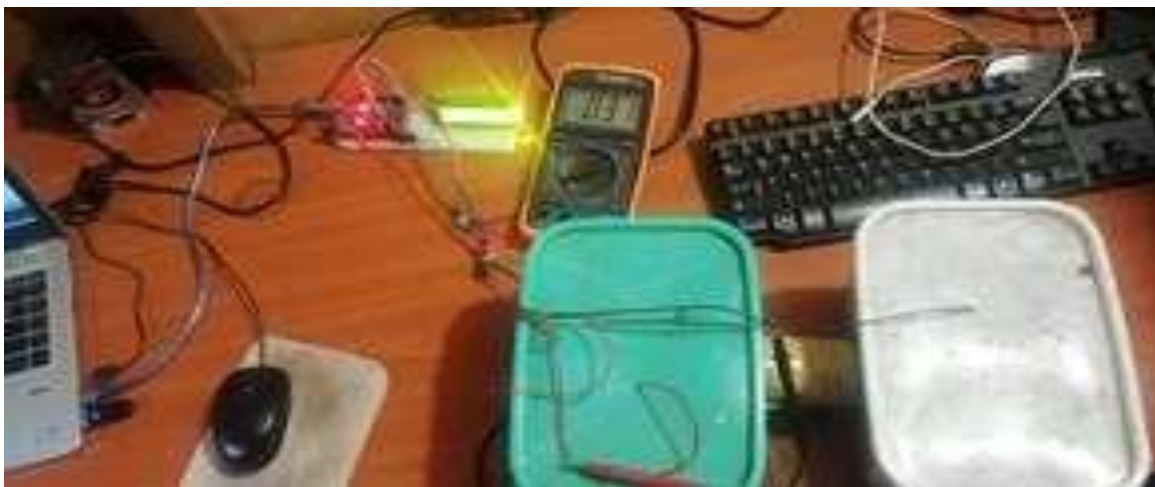
Figure 3.13: Arduino potential difference and current MFC monitoring gadget
