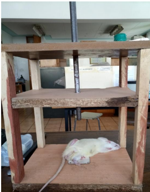
Figure 3. Device for inducing fractures
