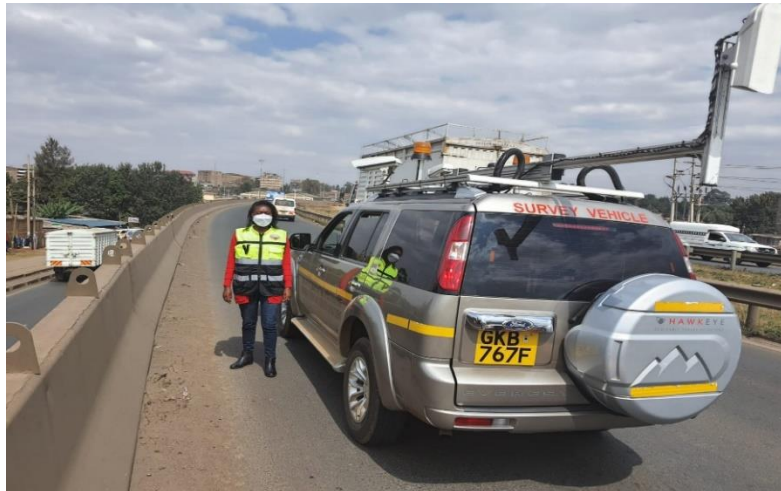
Figure 3-5: surface condition survey using Hawkeye 2000
