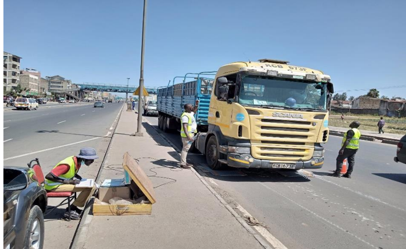
Figure 3-3: Axle load survey
