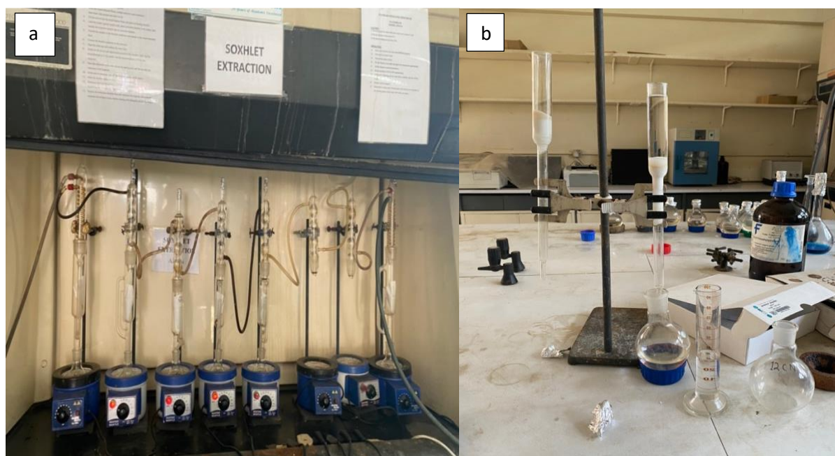
Figure 3.3: Soxhlet extraction of the soil samples (a) and clean-up of the extracts (b).
