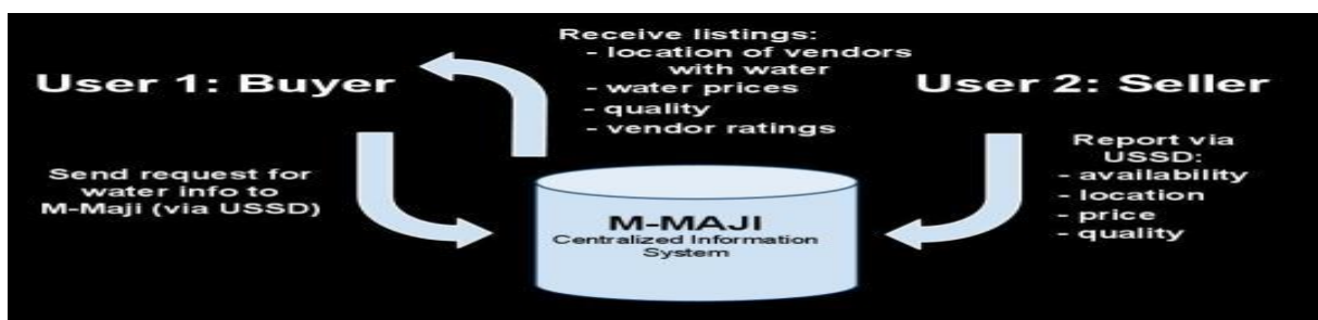
Figure 2.8: Illustration of how M-Maji works in Kibera Slums. Source: Umande Trust, 2020
