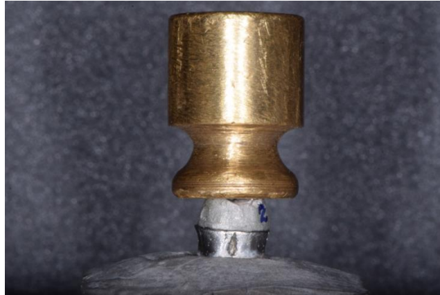
Figure 15: Seating of the cast-metal crown copings on the metal die preparation
