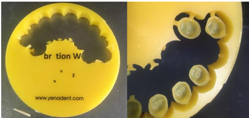
Figure 10: Yenadent® CAD-CAM wax block with the milled wax patterns
