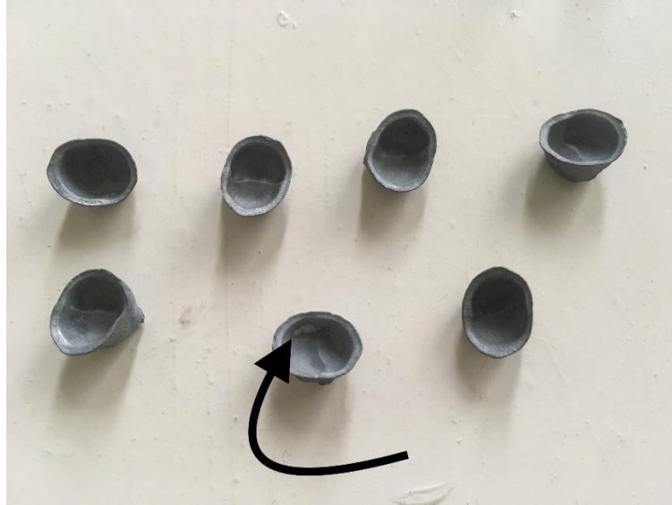
Figure 18: Cast-metal crown copings sectioned out from the casting formation. Arrow shows example of extensions that had to be modified with a bur before seating onto the master metal die.
