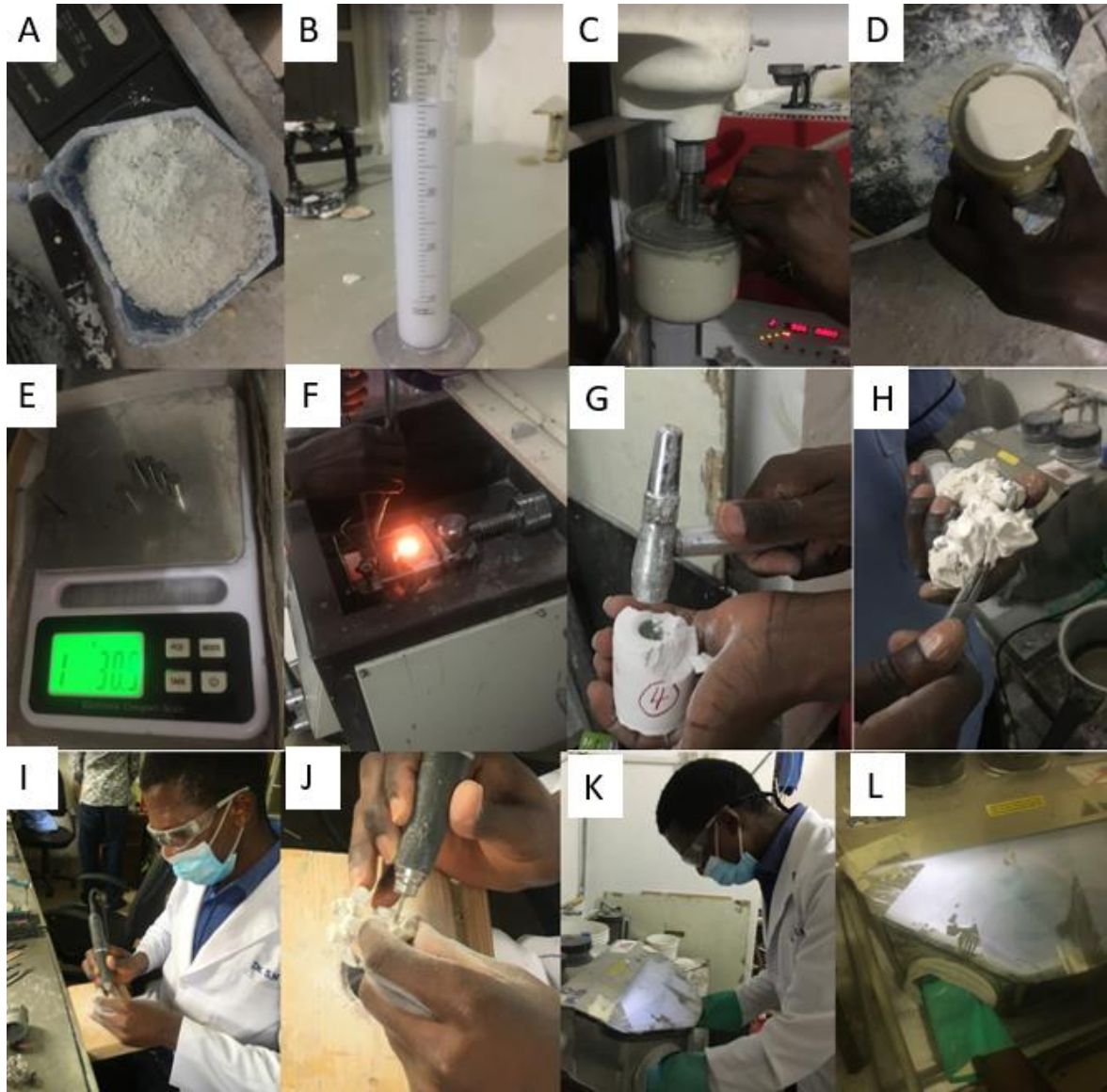
Figure 13: Investment, casting and divesting processes. (A) and (B): Measurement of the powder and liquid for Castorit super C phosphate bonded investment materials for casting the crown copings in the C-mr group. (C): Mixing the powder and liquid using a vacuum mixer. (D): Pouring the investment material into the rubber casting ring, while holding it against a dental vibrator. (E): Measurement of the weight of the cobalt-chromium metal ingots. (F): Placement of the investment mould into the induction casting machine after the wax burn-out procedure and melting of the metal alloy ingots. (G) Divesting the castings in the C-mm group using a hammer as is done by laboratory technologists in Nairobi, Kenya. (H) Divesting the copings using forceps as is recommended by the various manufacturers of the investment materials. (I) and (J): Removal of investment material from the fitting surface of the crowns. (K) and (L): Sand blasting using 50 \mu\text{m} alumina particles.
