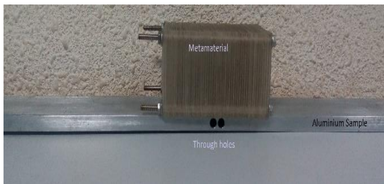
Figure 4. 11. Photograph of straight channel metamaterial positioning on top of defects
