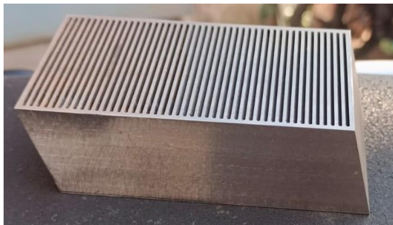
Figure 4. 12. Photograph of inclined angle channel metamaterial
