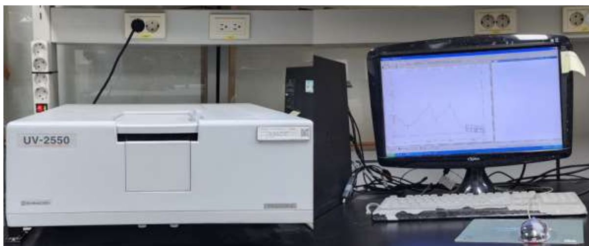
Figure 4.4: Photographic illustration of the optical absorption spectra measurement using the UV-visible spectrophotometer connected to a computer.
