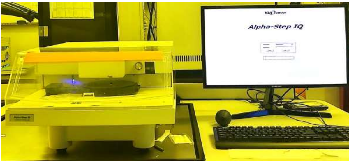
Figure 4.5: Photographic demonstration of Alpha Step-IQ surface profiler measurement system.
