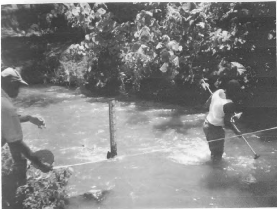
Plate3.2: Note a single staff gauge in the river and the measurement fo gauge height and river discharge simultaneously to generate a rating curve for the station IJC 19 – Kimugu - Kitenges
