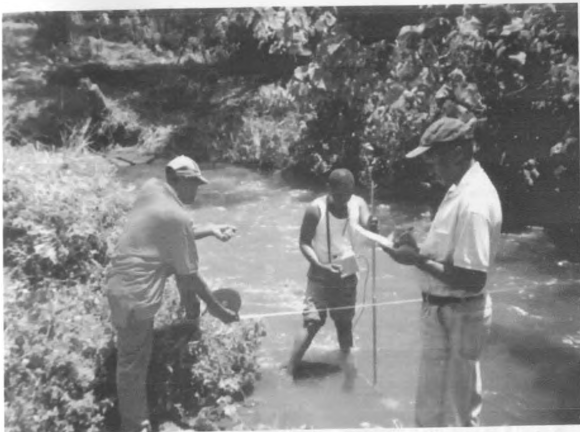
Plate 3. 1: Note the Mid Section method of river gauging, the researcher taking records as the research assistant in the middle, reads the meter counter.
