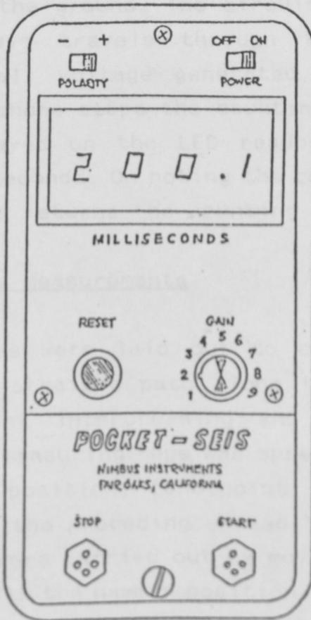
Fig 4.1 POCKET-SEIS ENGINEERING SEISMOGRAPH.
