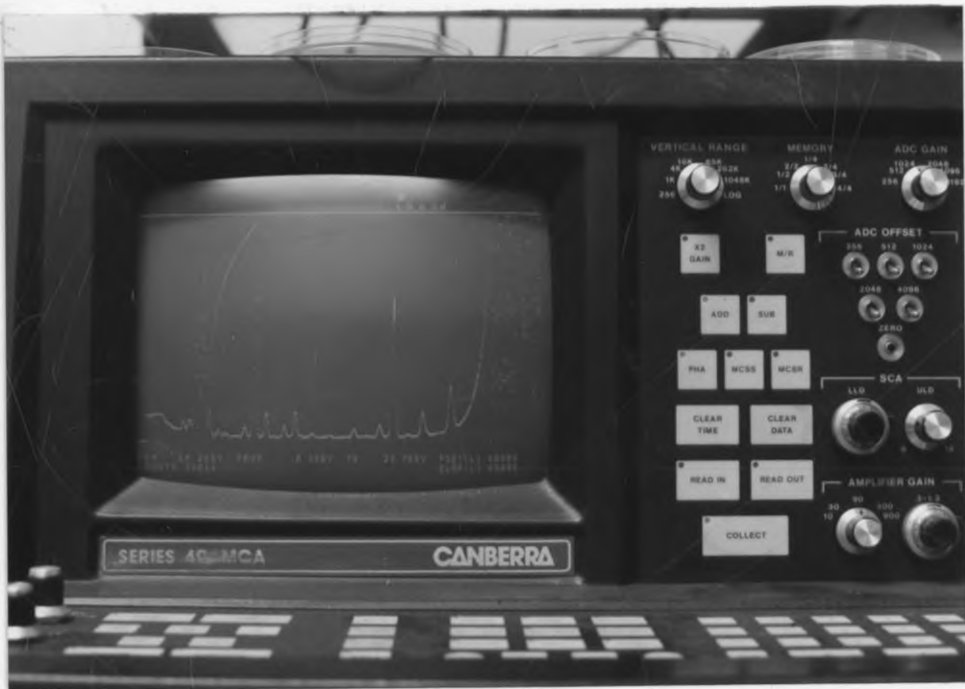
Plate IX (b) A CRT Spectral Display of a plant sample as displayed on the MCA, shows range of excitation from 0.3 KeV to 22.7 KeV with the ^{109}\text{Cd} Source.
