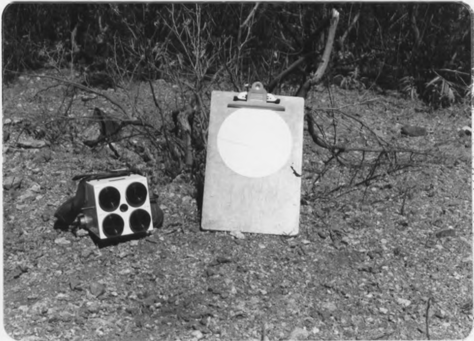
Plate VIII (b) The Portable Field Radiometer, with a white target for measuring energy incident upon an object.
