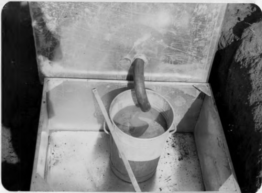
Plate 3. Storage tank and the drum inside with small storm awaiting sampling (Photo taken on 8/4/89).
