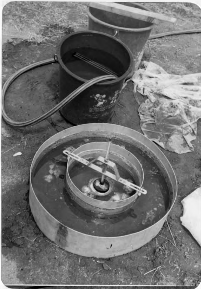
Plate 8. Experimental set-up for determining infiltration characteristics of sealed soils under different treatments (Photo taken in June 1989).
