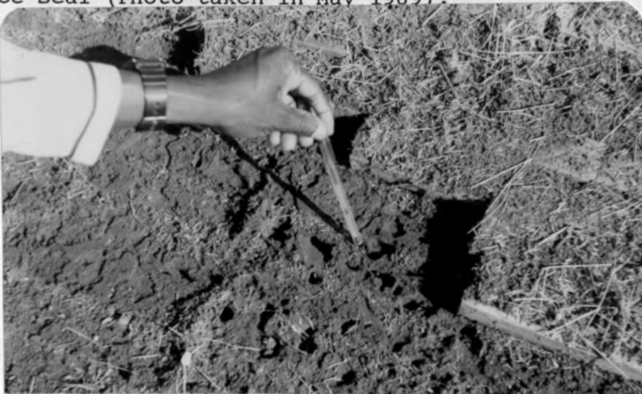
Plate 7. Tunnels created by termites after the cover material is removed (Photo taken in May 1989).
