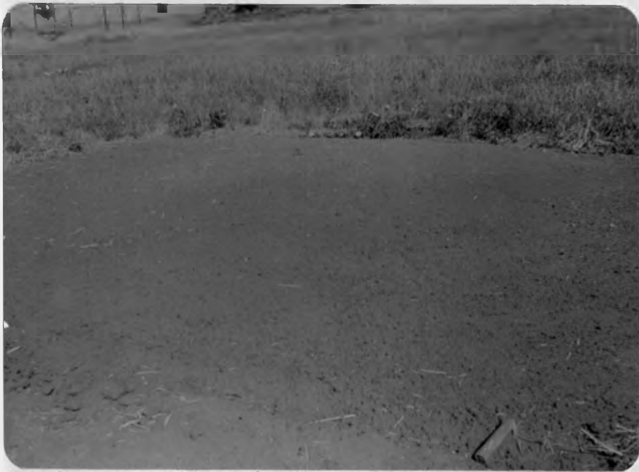
Plate 5. Land prepared for infiltration tests. Seal is broken and land levelled (Photo taken in April 1989).
