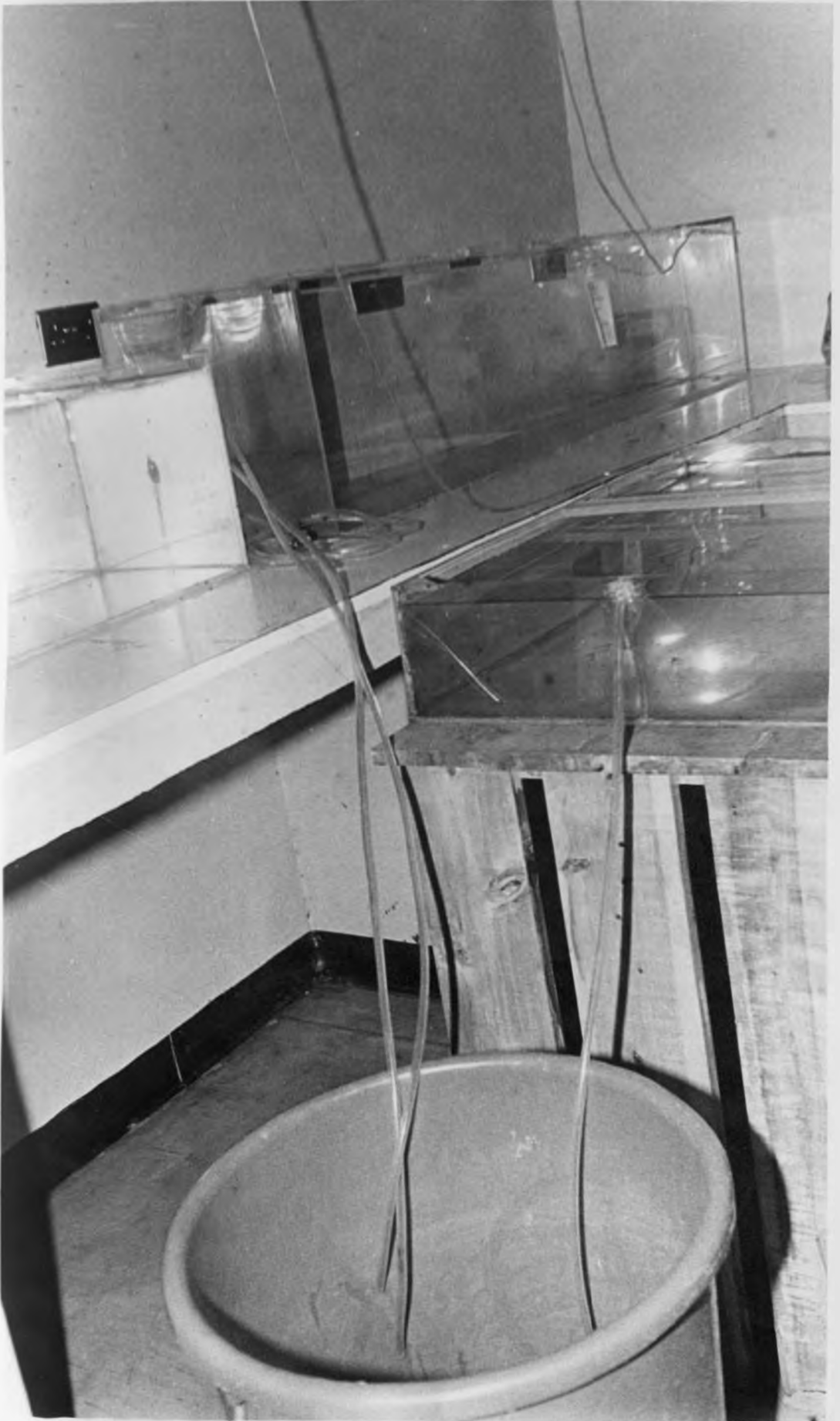
Figure 4.3. COLLECTION OF EFFLUENT FROM MODEL PONDS
