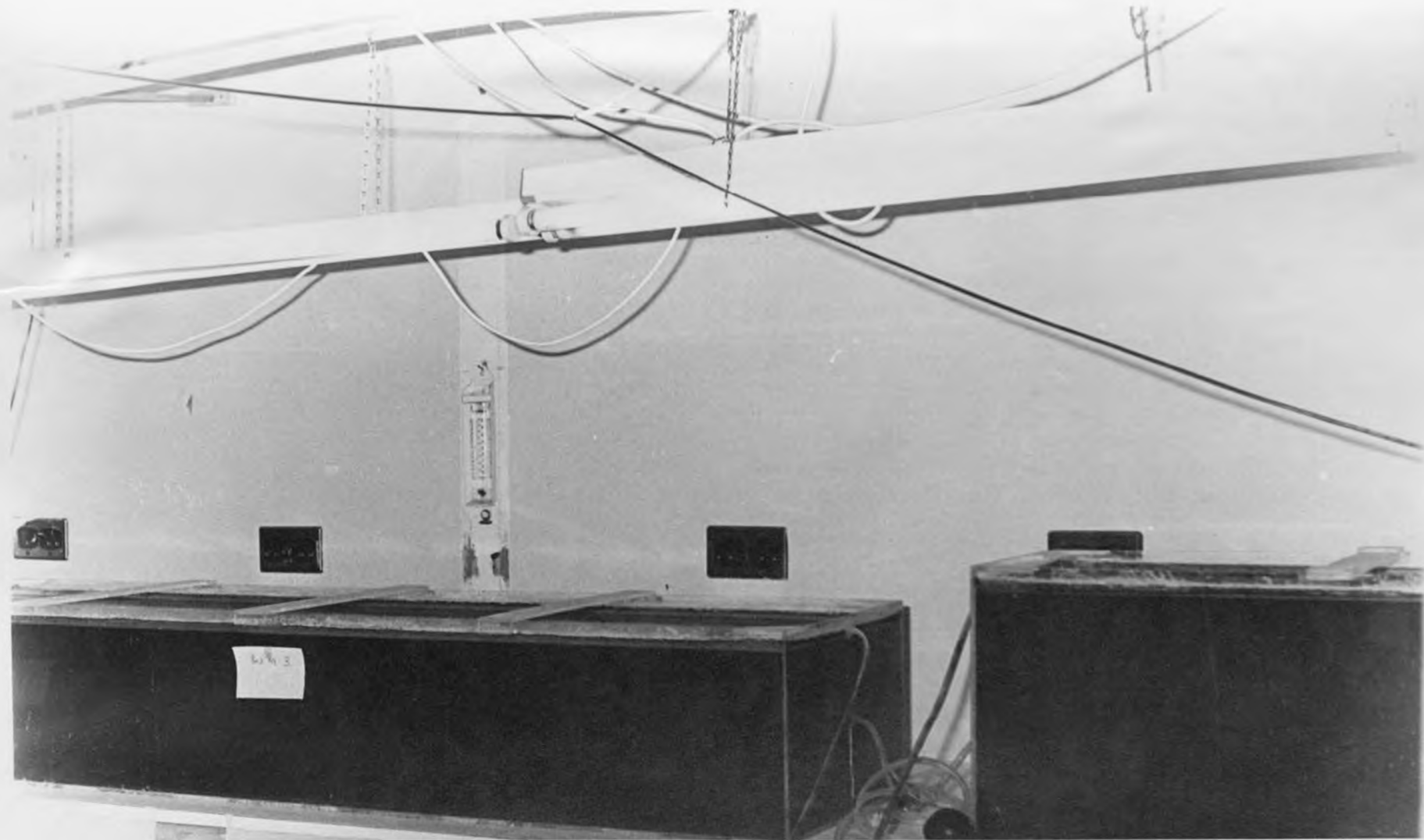
Figure 4.5. ARRANGEMENT OF MODEL PONDS AND LIGHTING SYSTEM
