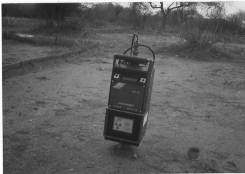
PLATE 3: The Neutron probe used to measure soil moisture.
