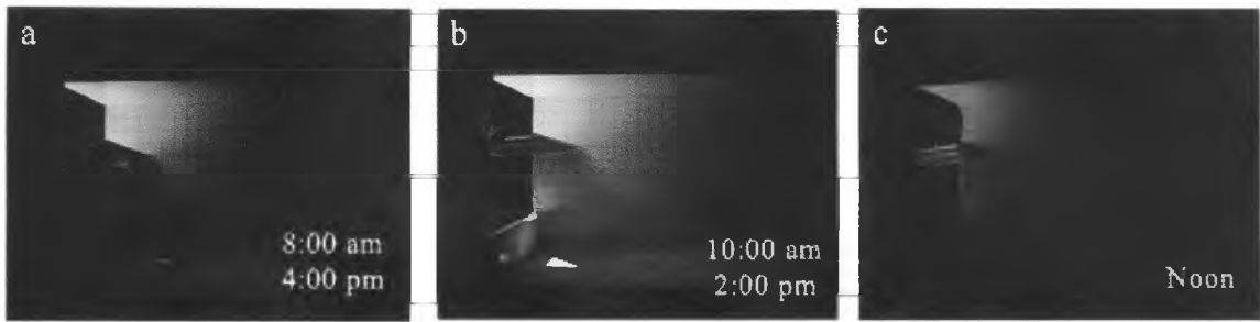
Figure 36: The daylight distribution for a North/South oriented opening at (a) 8am and 4pm, (b) 10 am and 2pm, and at (c) noon.
