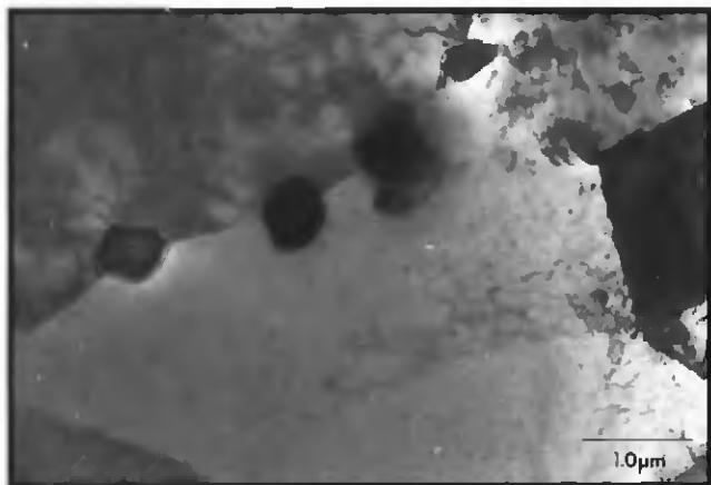
Fig. 5 — A TEM micrograph showing an example of incoherent grain boundary precipitation in the HAZ 2 mm from the weld interface.
