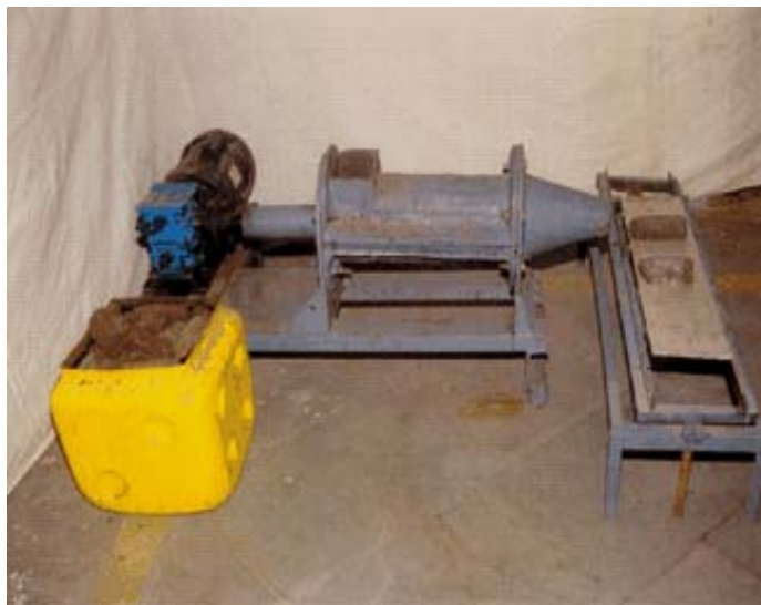
Figure 5. A simple electrical powered briquetting machine.
