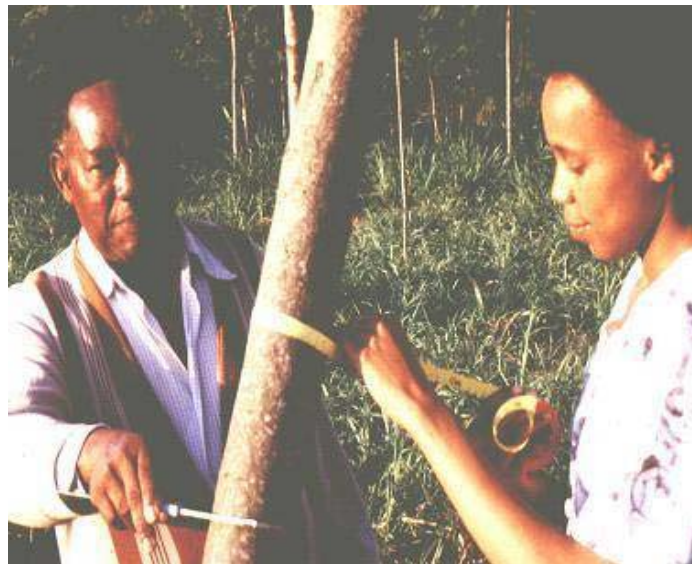
Figure 1. Measuring tree diameter with a dial caliper (left) and a diameter tape (right).
