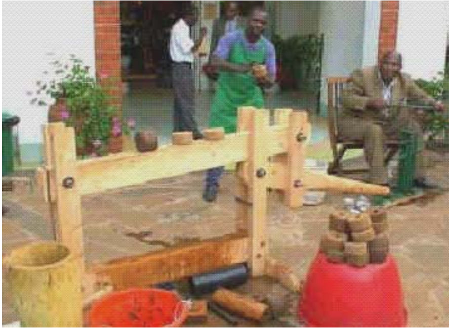
Figure 3. Two briquetting devices developed in Kenya that were displayed at a FORMAT event by the Millennium Fuel Project (left) and the Kayole Environmental Management Association (right).
