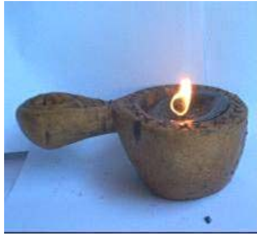
Figure 3. A simple wick lamp that burns using the avocado oil.
