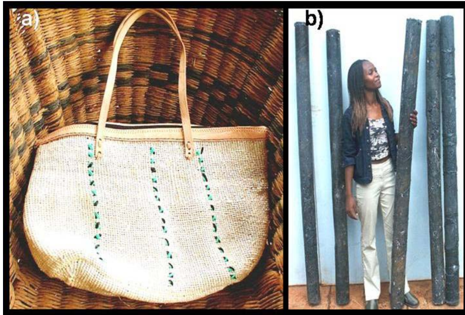
Figure 4. Plastics recovered from sorted domestic wastes may be recycled into a wide range of useful products such as handbags (a), hats and waste bins woven from clear polythene or fence posts (b) and roofing tiles remolded from darker plastics. The photographed products were produced by the Kayole Environmental Management Association, Nairobi.
