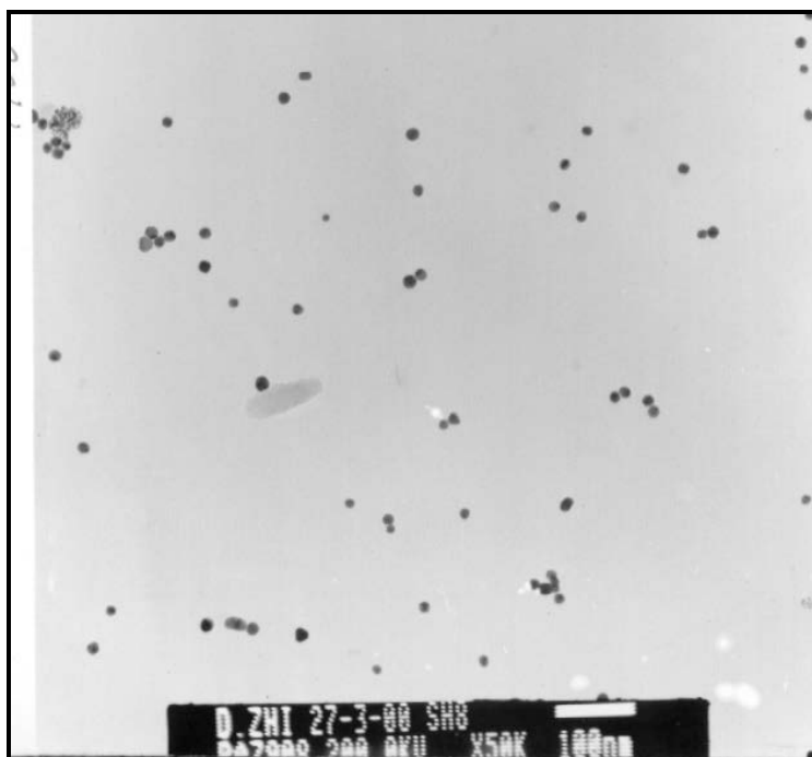
Figure1: TEM of a freshly prepared Gold Colloid ( \lambda_{\text{max}} = 520 \text{ nm} ).
