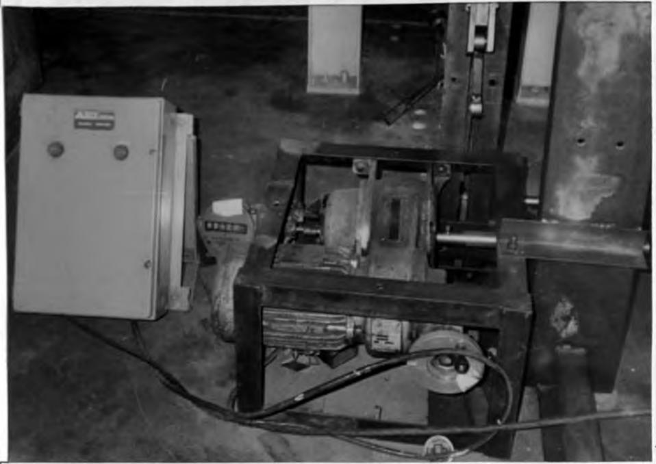
PLATE (3.1) THE MOTOR AND GEAR BOX ASSEMBLY.
