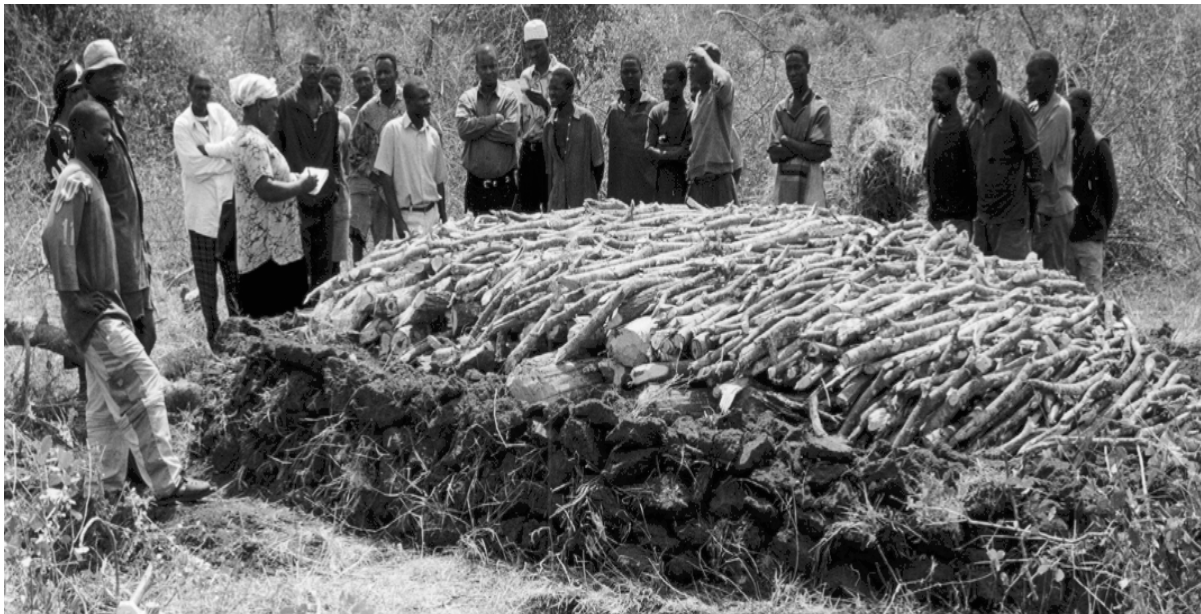
Earth mound kilns: Efficiency has been reported to range from 8-15 per cent.
