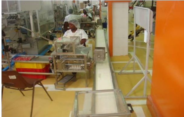
Figure 4-18: Main Cube conveyor
