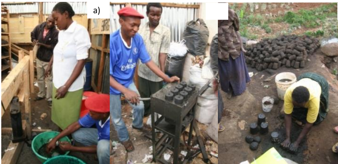
Figure 4.1. Pressing fuel briquettes using (a) wooden manual press (b) metal manual press and (c) molding in recycled plastic container
